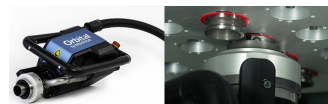
A portable Novator orbital drilling machine and a close-up view of the drill jig and bushings to which the machine is clamped for each hole. RFID tags in the drill plate and machine ensure only the correct hole is drilled.
